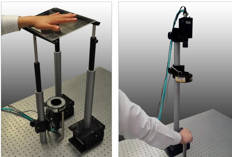
Image acquisition system of the palm and back of the hand vein distribution.
